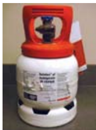
This is a HFO 1234yf refrigerant cylinder, first seen in Manitoba in 2013. They are half the size of a typical ODS cylinder, as its introductory price is substantially higher than many HFCs.
