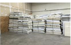
Pictured above: foam bundled and ready to ship for processing - capturing the HCFCs. Compressors from units dripping oil into a safe recovery tub.
