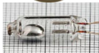
Contractors and the public are encouraged to properly dispose of used mercury switches.
